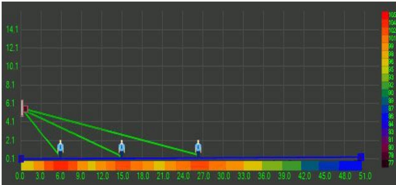
Figure 1: 3 SPL distribution map for preset positioning
